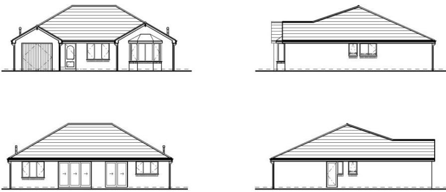
Left – Elevations of the proposed house type, to give an impression of the proposed materials and form of the property
